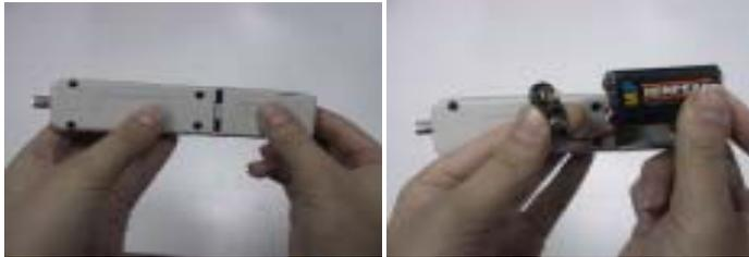
2. Remove the protective covers from the fiber connector.
